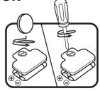
Replace the battery cover and tighten the screw to secure the battery cover.
